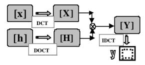
Figure 2: Linear filtering or convolution in the DCT domain.
